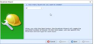
3. Click **Next** to display the next page. Change Layer 1's thickness to 8 m and (if necessary) its soil type to "Sand" and weight density to 20 kN/m<sup>3</sup>.
