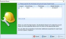
Click Next to display the next page. Change the sand's Internal friction to 35° but leave its Cohesion unchanged at 0 kPa. This is the sand's peak angle of friction.
