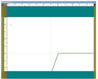
"6 m high slope", change its **Height** to 6 m, and its **Main Slope** to 70°. The **Breadth** changes to 2.18 m. The new dimensions of the slope are reflected in the **Drawing Board**.
